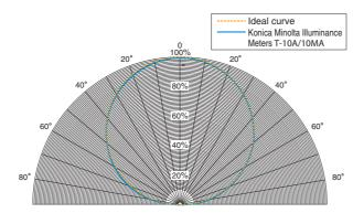
Since the brightness at the measurement plane is proportional to the cosine of the angle at which the light is incident, the response of the receptor must also be proportional to the cosine of the incidence angle. For Konica Minolta Illuminance Meters T-10A/10MA, the cosine response f2 is within 3%.
